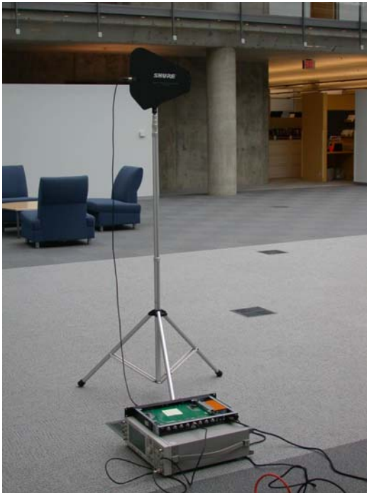
Photo 1. 100mW Transmitter into +6dBi Directional Antenna Equipment Setup
