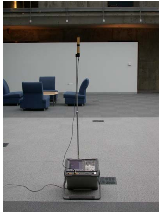
Photo 2. Spectrum Analyzer with 0dBi Omni-directional Antenna Equipment Setup
