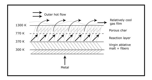
For the shuttle RSRM, the throat insert (C cloth phenolic) regresses  $\sim$  1 inch/120 sec, and the char depth is  $\sim$  0.5° inch/120 s.
