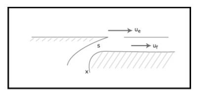
Assume we know the flow rates  $m_{\text{\tiny C}}$  and  $m_{\text{\tiny F}}$  , where  $m_{\text{\tiny C}}$  is the "core" flow and  $m_{\text{\tiny F}}$  the "film" flow. We also know the fully-burnt temperatures and molecular weights (  $T_{\scriptscriptstyle C}$  ,  $T_{\scriptscriptstyle F}$  ;  $M_{\scriptscriptstyle C}$  ,  $M_{\scriptscriptstyle F}$  ).
