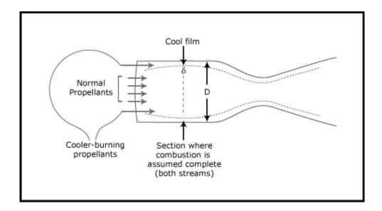
For application of data on slot-injected films, we need to define the initial film thickness s, velocity  $u_{\!\scriptscriptstyle F}$  , density  $\rho_{\!\scriptscriptstyle F}$  , or at least mass flux  $u_{\!\scriptscriptstyle F}\rho_{\!\scriptscriptstyle F}$  .
