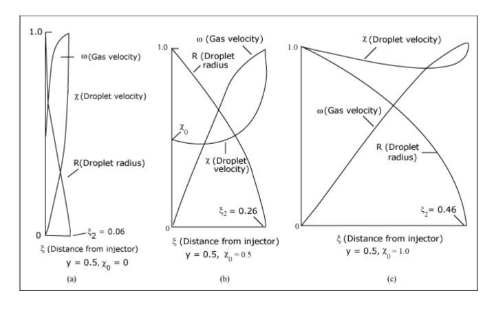
Evolution of evaporating droplet size and velocity. Here the reference  $v_{ref}$  for velocity is that of the gas after complete evaporation, and for length,  $l_{ref} = 2 \, v_{ref} \, \tau_v$
