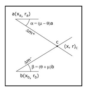
(1) Calculate  $\left(x,\,r\right)_{\!c}$  from the angle  $\left(\mu-\theta\right)_{\!a}$  ,  $\left(\mu+\theta\right)_{\!b}$
