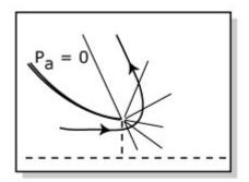
Actually, one starts from some high M<sub>e</sub>>1, so the actual turning is through  $\omega_{_{\infty}}-\omega \left(M_{_{e}}\right)$ , not  $\omega_{_{\infty}}$ , even in a vacuum:
