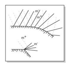
Consider a <u>uniform</u> region; the flow from it enters some disturbed region, like a wall turning. One of the m families originate in the uniform region (m<sup>+</sup> in example) and carries a <u>constant</u> invariant, e.g.  $\vartheta + \omega = \vartheta_o + \omega_o$  everywhere downstream. Along one of the <u>other</u> characteristics (m<sup>-</sup> here), we carry a constant (which varies from ch. To ch. of that family); we can evaluate it at the wall, for instance
