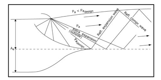
Pressure forces from hot-gas bathed surfaces are the same as at design. Net thrust is increased because the  $P_a$  contribution  $P_aA_e$  is reduced:
