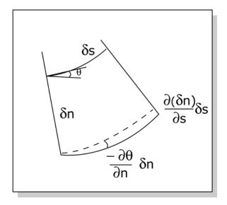
$$\frac{1}{\rho}\frac{\partial \rho}{\partial s} + \frac{1}{u}\frac{\partial u}{\partial s} + \frac{1}{r}\frac{\partial r}{\partial s} + \frac{1}{\partial n}\frac{\partial \delta n}{\partial s} = 0$$
