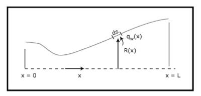
The local heat loss per unit area is  $q_w = \rho u c_p \left( T_{aw} - T_w \right) S_t$ , and using  $\dot{m} = \rho u \pi R^2$ , the integrated heat loss is
