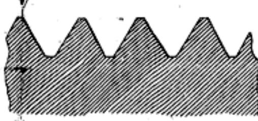
**29. The significance of the Seller's screw thread standard is that each of us can go to a hardware store today, purchase nuts and bolts, and put them together. We don't need to take a Fundamentals of Mechanical Engineering Laboratory to put nuts and bolts together. It just works.**
