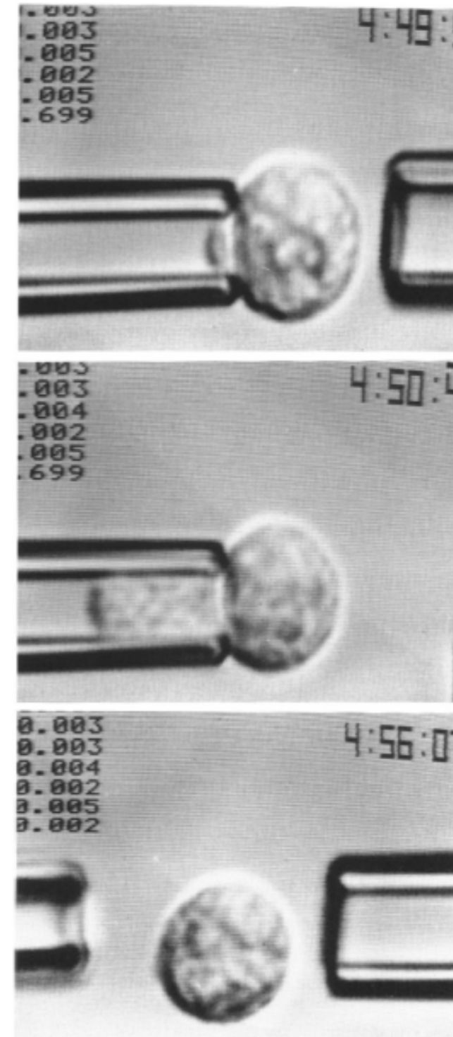
FIGURE 1 Sequence of video micrographs of a blood granulocyte aspirated into a 3.5 \mu\text{m} caliber pipet: (a) first, formation of a hemispherical cap at the threshold pressure with no further flow; (b) next, the extent of flow after the suction was elevated above the threshold for a fixed time period then returned to the threshold value; and (c) recovery of the cell to its initial spherical form after release from the pipet.
