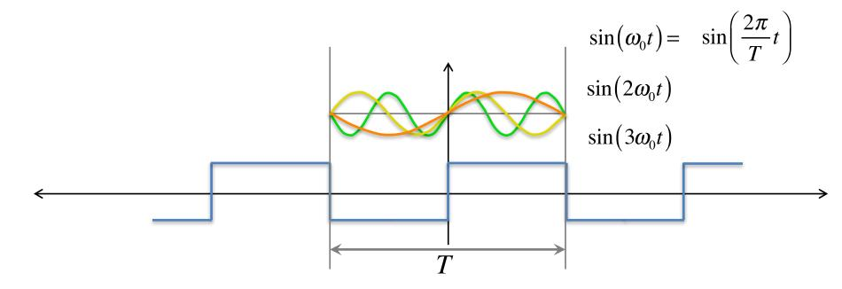
$y_{odd}(t) = \sum b_n \sin(n\omega_0 t)$  $y_{odd}(t) = b_1 \sin(\omega_0 t) + b_2 \sin(2\omega_0 t) + b_3 \sin(3\omega_0 t) + \dots$ Why is there no DC term here?
