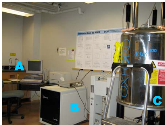
Figure 1 NMR Equipment: (A) Computer Workstation, (B) NMR Console, generates and receives RF, (C) NMR Magnet.
