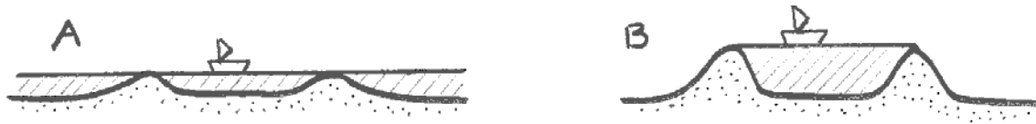
Figure 5-49. The stage of a flood flow for a given flood discharge. A) Before building of levees. B) After building of levees.
