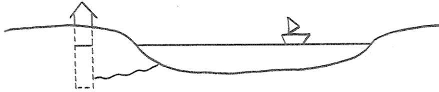
Figure 5-2. A stream-gauging station.
