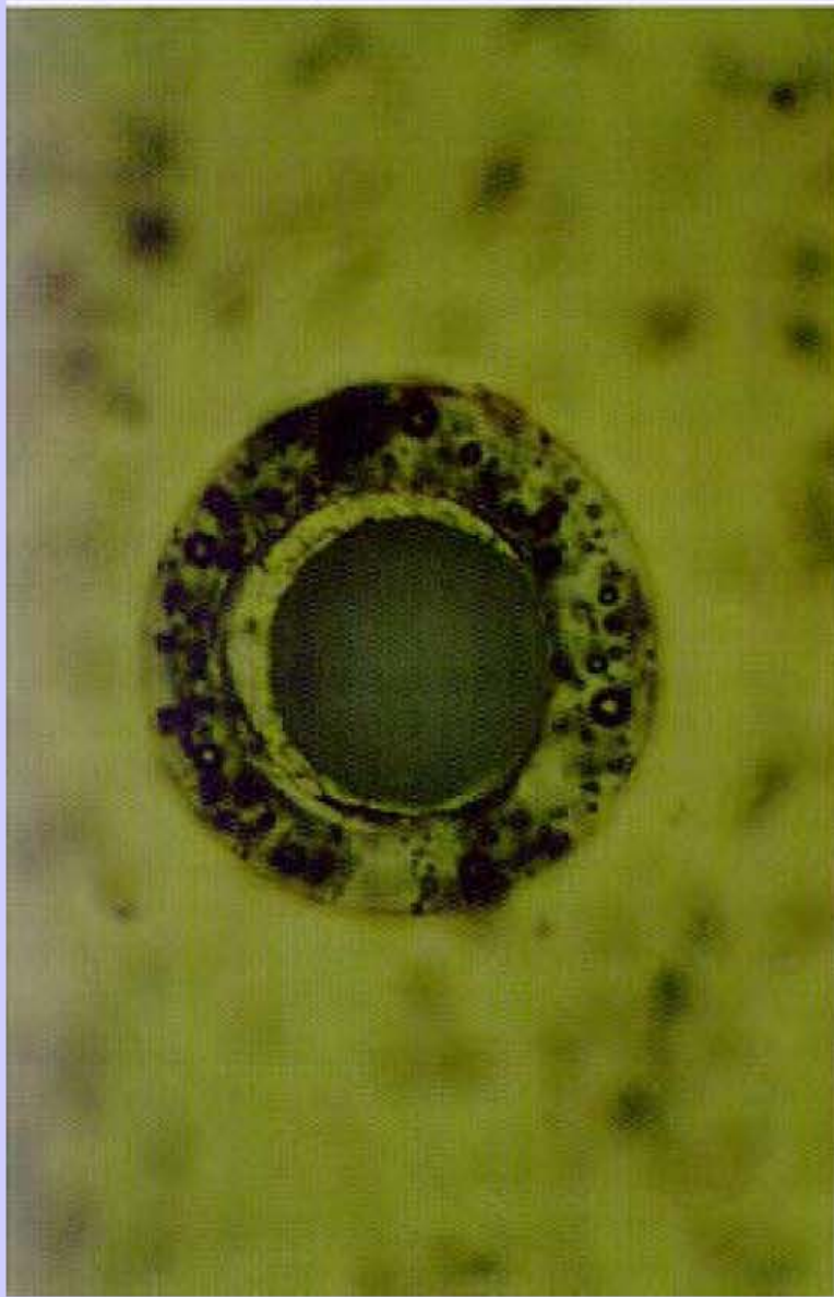
Photograph of hollow glassy fly ash particle (0.01 cm D)
