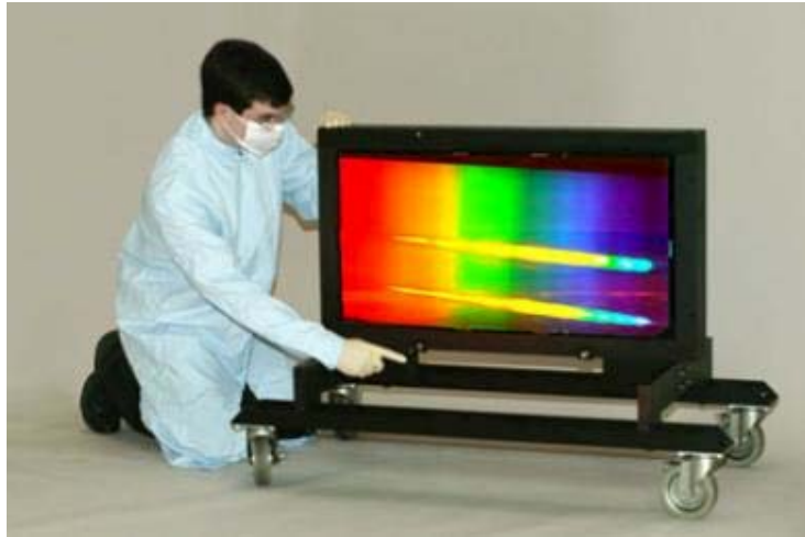
One of world's largest multilayer dielectric diffraction gratings
