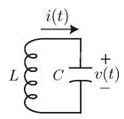
capacitor charge: q(t) = Cv(t)
