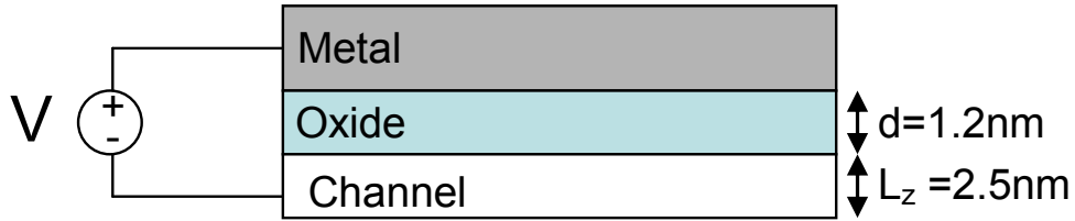
Fig. 2.28. A simple model of a modern transistor.
