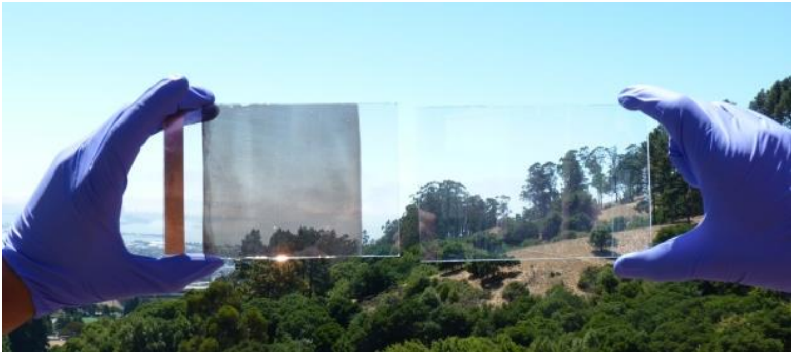
Photo of heat- and light-blocking film on glass © Anna Llordés, Lawrence Berkeley National Lab. All rights reserved. This content is excluded from our Creative Commons license. For more information, see http://ocw.mit.edu/help/faq-fair-use/ .
