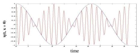
4. A wave train (red line) constructed with two waves having similar frequency/wavenumber components. This wave appears to be beating. The blue line shows the "envelope" or group outline.
