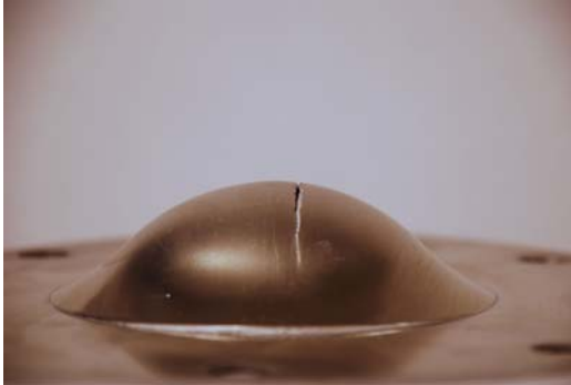
Fig. 2-30 A view of the fractured disk
