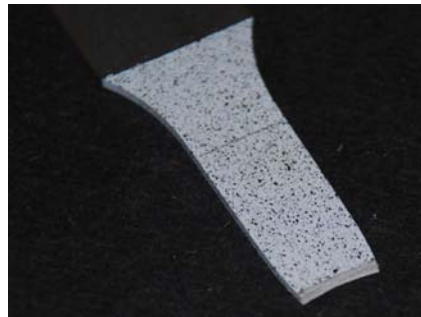
Fig 2-16 Necking occurs in tensile tests
