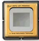
DLP 10^6 micromirrors, each 16\mu\text{m}^2 , \pm 10^\circ tilt (Hornbeck, Texas Instruments DMD, 1990)
