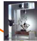
First transistor made in 1947 by Shockley, Bardeen, and Brittain at Bell Labs.
