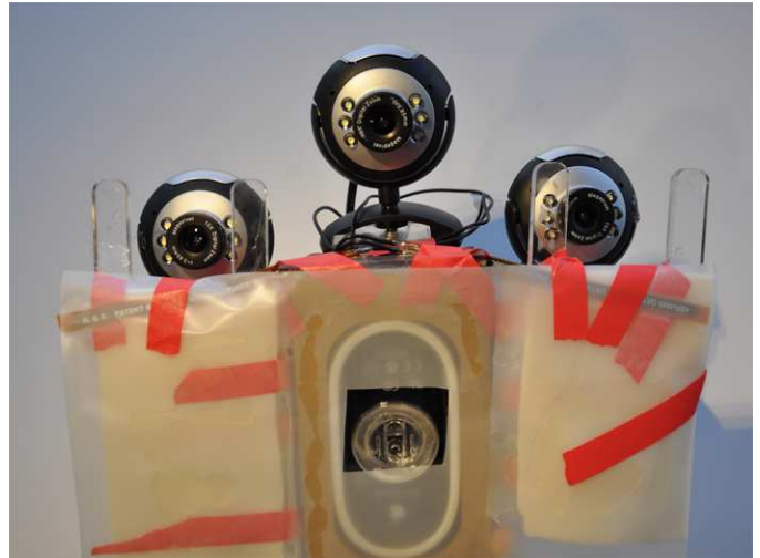
Figure 5: The underside of the scanner. Here the optical mouse is visible along with the bend sensors.
