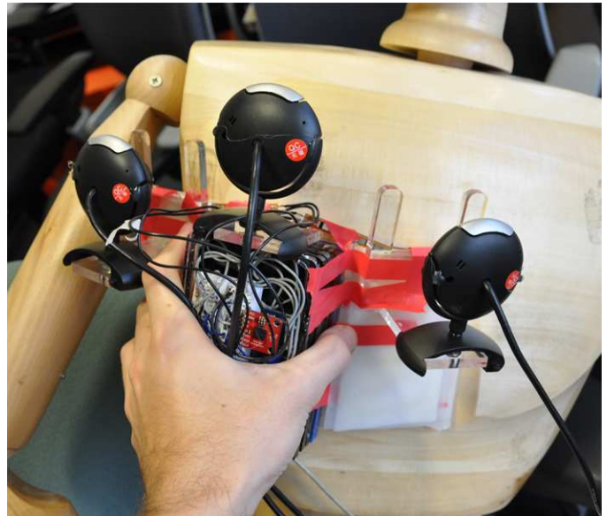
Figure 6: The final prototype in action. Note that the cameras can bend to conform to the shape of the object being scanned.
