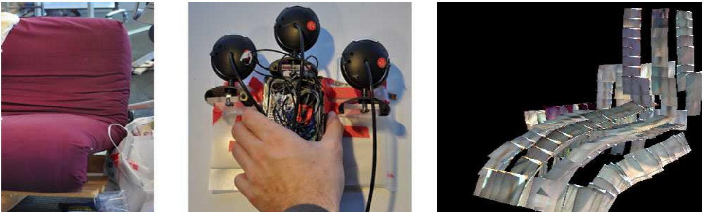
Figure 1: Left: Input into our system, a chair. Center: An articulated 3D mesh scanner. Right: Our result, a scanned chair.
