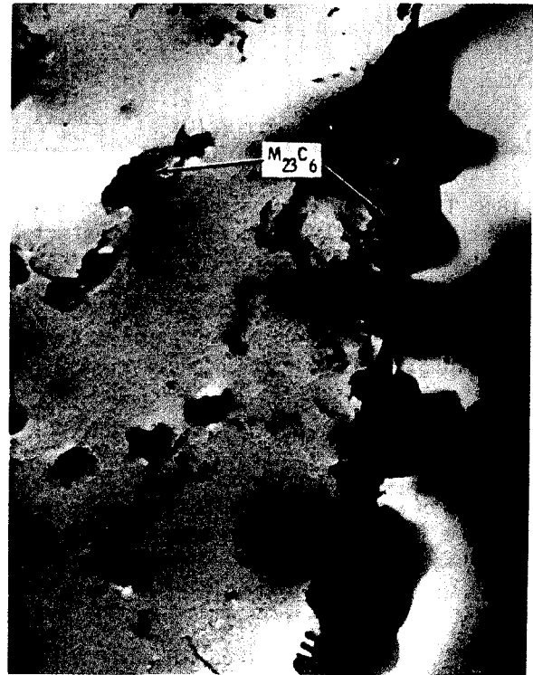
Fig. 18.7 Nearly continuous M_{23}C_6 precipitation along grain boundary of solution-treated type 316 irradiated at 850°C to 5.1 \times 10^{22} neutrons/cm 2 . [From H. R. Brager and J. L. Straalsund, J. Nucl. Mater. , 46: 134 (1973).]
