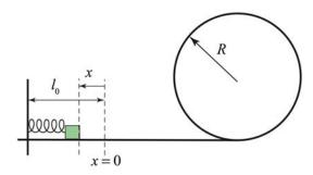
When the block reaches the top of the loop, the force of the loop on the block (the normal force) is equal to twice the gravitational force on the mass. How far was the spring initially compressed? Write your answer using some or all of the following: g, k, R, and m.
