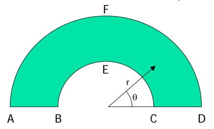
A potential difference V<sub>0</sub> is applied along the semicircular borders: the inner radius BEC is kept at potential  $V = V_0$ , while the outer radius AFD is kept at potential V = 0. a) Find the potential  $\phi$  everywhere on the plate, the electric field  $\vec{E}$ , the current density  $\vec{J}$  and the Ohmic resistance of the conductor R.
