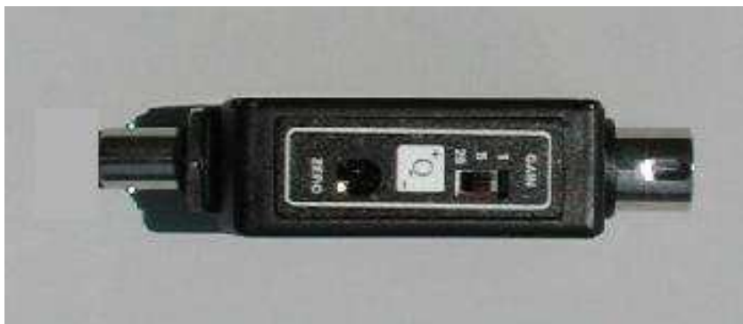
Figure 5: Gain and Zero Settings for the Charge Sensor
