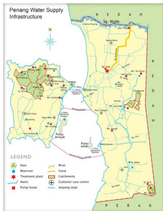
Figure 19. Penang Water Supply Infrastructure Map. Source: PBAPP, 2015.
