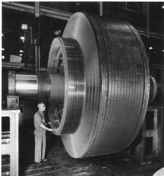
Fig. 4.1.26 A dc machine rotor (armature). Note the large number of slots and commutator bars. (Courtesy of Westinghouse Electric Corporation.)
